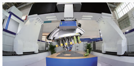
Gantry Type Filament and Tape Lay-Up Machine for Carbon Fiber Composite Material with Ground Railways, Model GATL40/L120
